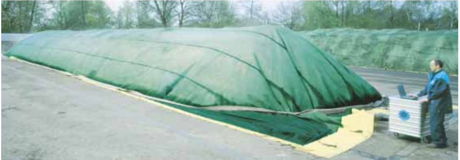
Sophisticated technology – clamp with mobile aeration equipment and Gore cover for rapid composting
